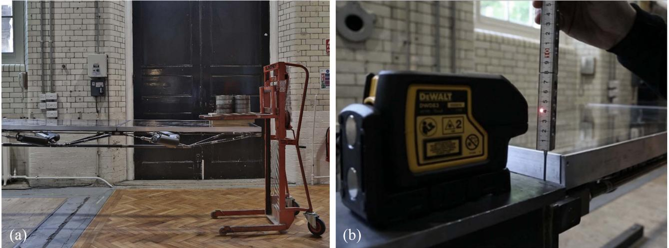
Figure 18. (a) Load test; (b) node displacement measurement.
