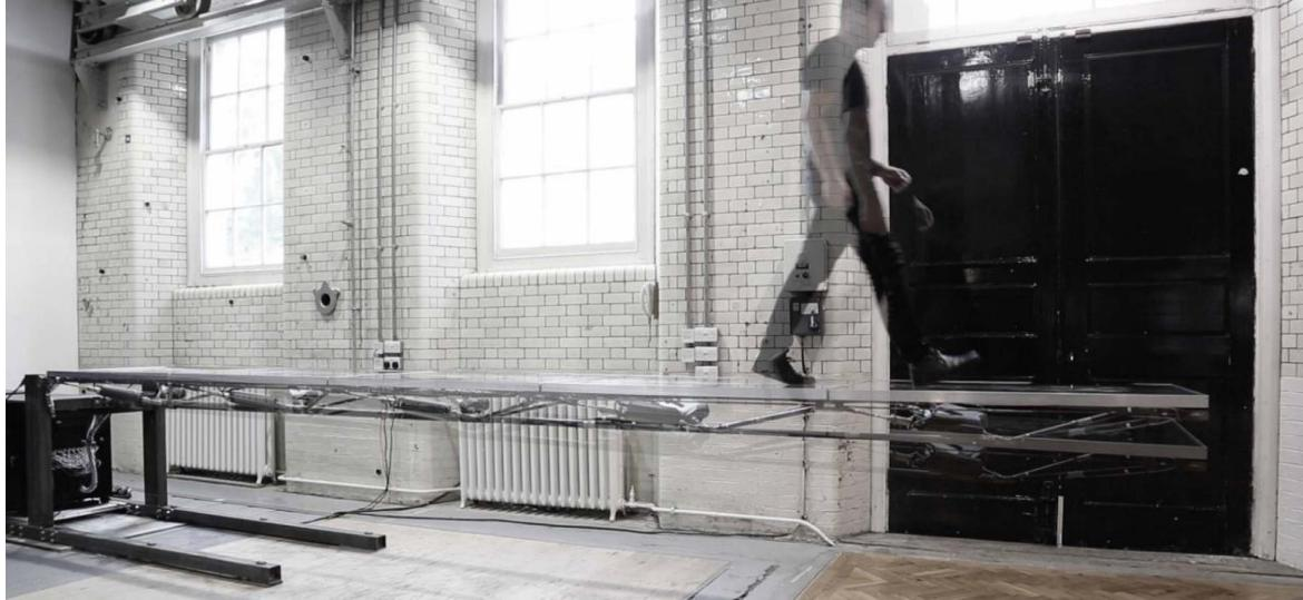
**Figure 24.** Person (70 kg) walking, comparison deformed (transparent) and controlled shape.
